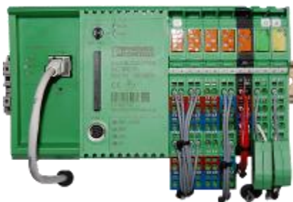
Fig. 5: Inline-Controller ILC 350 PN with Flash Memory card and additional analog I/Os
