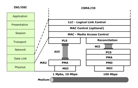
AUI - Attachment Unit Interface MDI - Medium Dependent Interface MII - Medium Independent Interface MAU - Medium Attachment Unit
