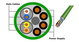
Symmetrical because the potential difference to the reference ground is 0 V in an ideal case. To transmit a signal, two wires are twisted together as a signal pair.
