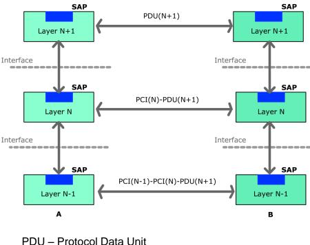
PDU – Protocol Data Unit PCI – Protocol Control Information According to the ISO/OSI reference model, communication operations can be divided into seven layers.
