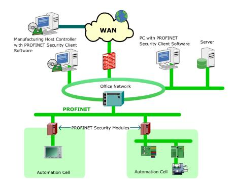
Each cell can be connected to the backbone through an entry point and are protected by using special security network components, such as switches or other security appliances.
