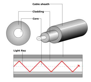
The light pulses are reflected totally and forwarded along the core. In order for data to be sent, the data signals are converted into light pulses by using LEDs or laser diodes.
