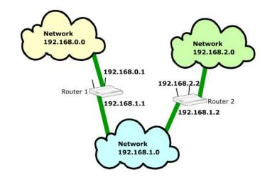
A router will look at the IP address of the data packet and determine, with the help of a subnetwork, whether it is within the same network or not. If not, it will forward the data packet to the appropriate network.
