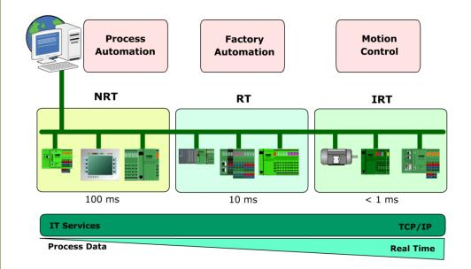
**NRT (Non Real Time)** for nontime-critical processes with use of standard TCP/IP and UDP/IP when transmitting data packets.
